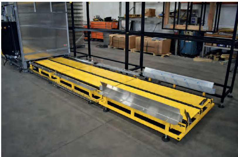
Below (L-R): Ska Fab's FHA 5000 depalletiser and inline high-speed single filing conveyor
